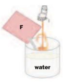
The product should be mixed in a forced action mixer or in an appropriate sized metal or plastic drum using a slow speed drill and a spiral paddle. The water should always be placed into the mixing vessel
